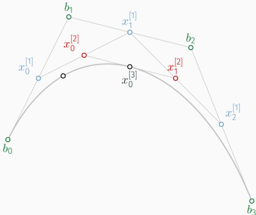
Same procedure for evaluation of  $\beta_3(\frac{1}{2}; b_0, b_1, b_2, b_3)$ .
