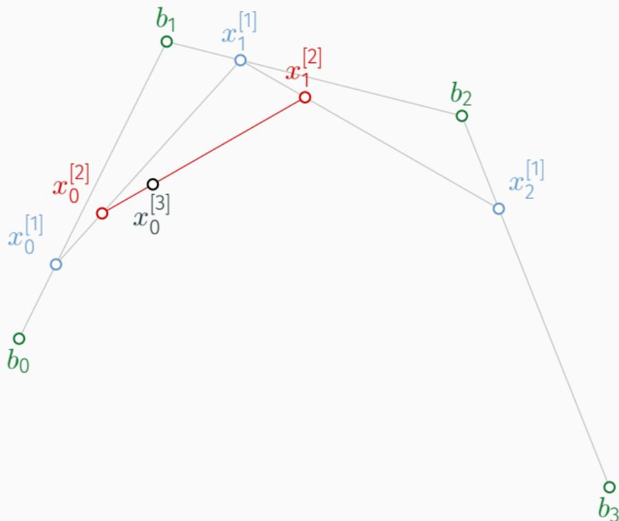
Repeat for the **last segment** to obtain  $\beta_3(\frac{1}{4}; b_0, b_1, b_2, b_3) = x_0^{[3]}$ .
