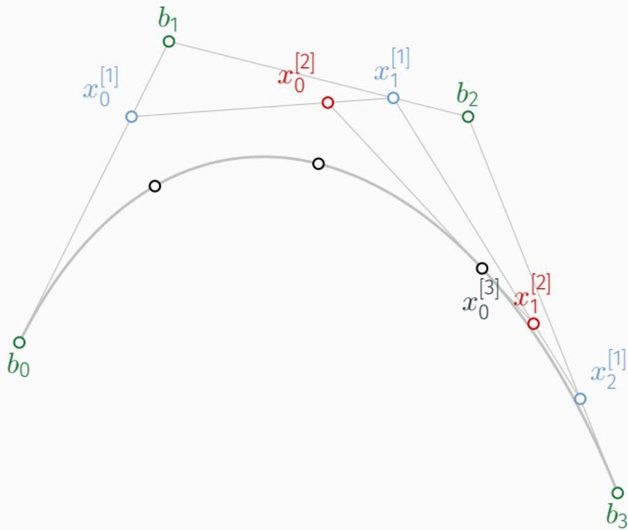
Same procedure for evaluation of  $\beta_3(\frac{3}{4}; b_0, b_1, b_2, b_3)$ .
