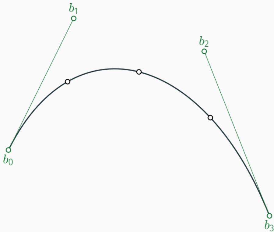
Complete curve  $\beta_3(t; b_0, b_1, b_2, b_3)$ .
